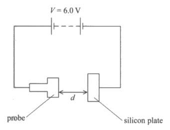
The relationship between the capacitance C and the distance d between the silicon plate and the probe is
