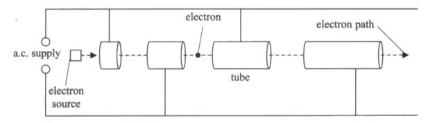
In the first part of the accelerator the drift tubes gradually increase in length, but at the end of the accelerator, the tubes are of the same length.
